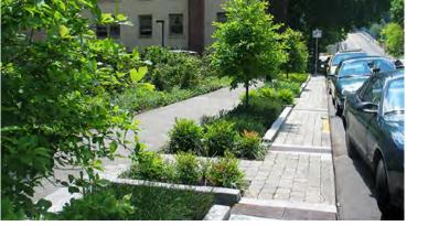
Figure 35: Precedents of microbioretention area. (Sources: Strada https://stradallc.com/2014/07/18/designing-stormwater-naturally/, (http://water.epa.gov/infrastructure/greeninfrastructure/images/Green-Street-Planters.jpg)
